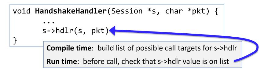
**Coarse CFI**: ensure that every indirect call and indirect branch leads to a valid function entry point or branch target
